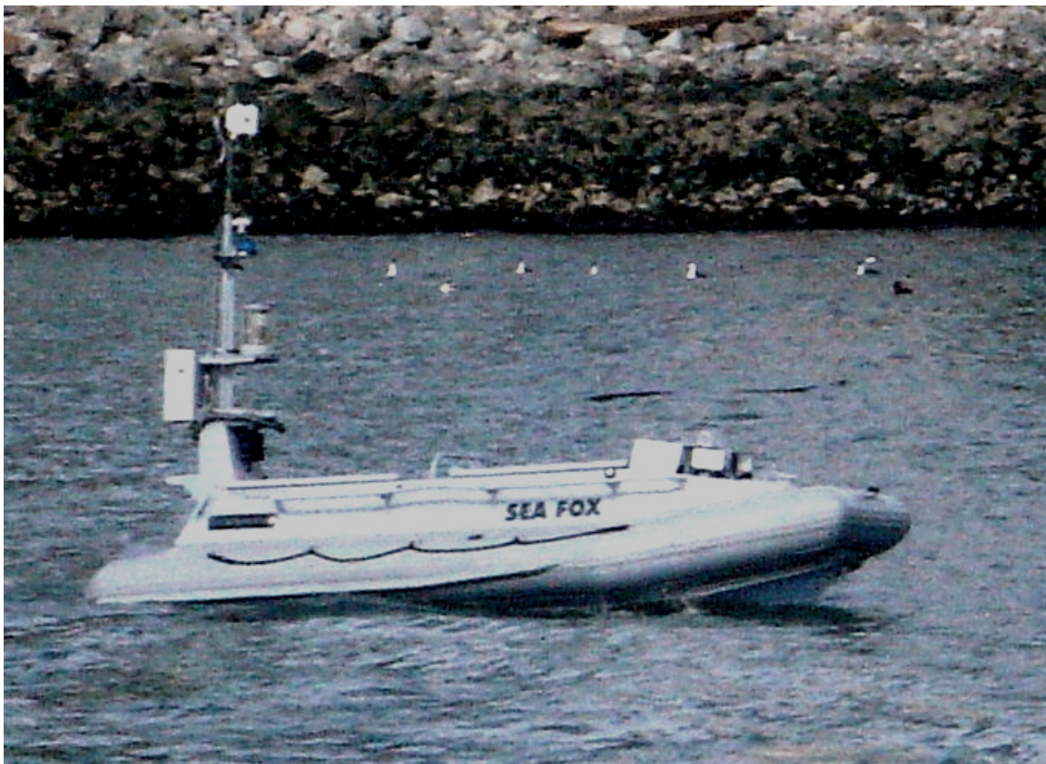
The “Sea Fox” remotely piloted boat fitted with Wave Relay mesh Wi-Fi and a radiation detector on day one.
