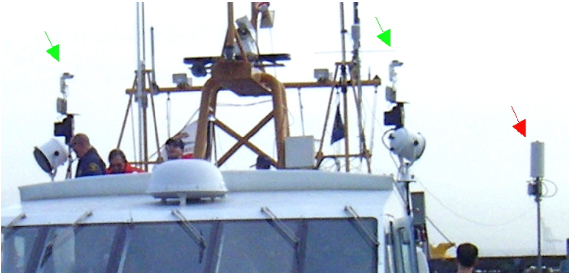
Broadband antennas used on the Alameda County Sheriff's boat for the day. Green arrows point out two geo-pointing 802.16 "ears", the red arrow point to the Wave Relay 802.11 antenna.
